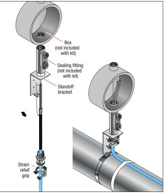
**Input Power Splice** (for power connection to two lengths of heater – additional kits required)
