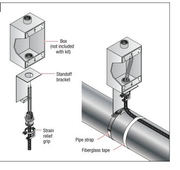
**Input Power Splice** (for power connection to two lengths of heater – additional kits required)
